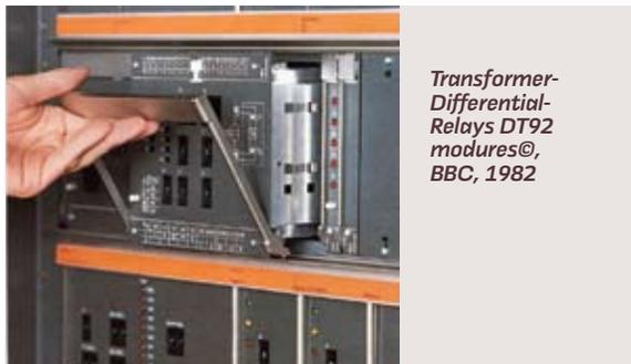
*Transformer-Differential-Relays DT92 modures®, BBC, 1982*
