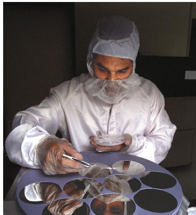
A Spectrolab, Inc. associate places wafers on platters to grow them into solar cells
