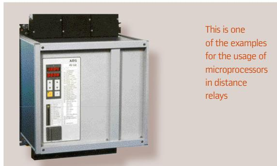
This is one of the examples for the usage of microprocessors in distance relays
